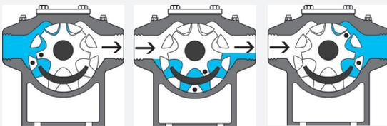
As shown in the illustration above, the gear pump with internal tothing results in almost no change in the flow direction through the pump, making this type of pump particularly well suited for pumping chocolate.
